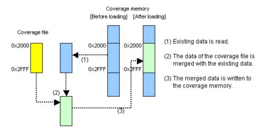
Figure 5.100 Schematic of load modes when selecting Merge
